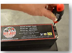
Remove the cover to the Room Silent Zone using an appropriate hex wrench or Phillips head screwdriver The unit will need to remain plugged in while making the adjustments.
