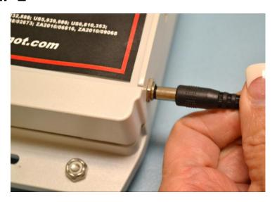
Plug the power adapter connector into the SPOT-Z.
