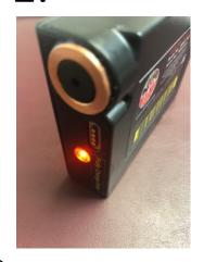
When off charge and active, the LED light will blink every 15 seconds to let the user know the PAD has power. If PAD is not blinking, charge. After the PAD is fully charged verify blinking. If unit is still not giving active indication, contact your dealer for repair information.
