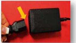
Placement of the module should be 2' from any metal wall or surface. Power up the unit using the 12V (3.3A) Power Supply. Connect the female plug into the power supply and plug into the outlet. A blue light on top of the unit illuminates when the unit is ON.
