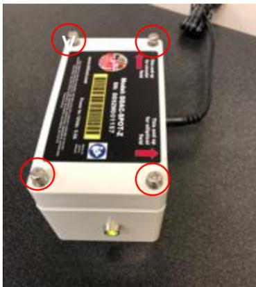
Remove the cover to the Spot Silencer using an appropriate Phillips head screwdriver. **The unit will need to remain plugged in (Powered) while making the adjustments.**
