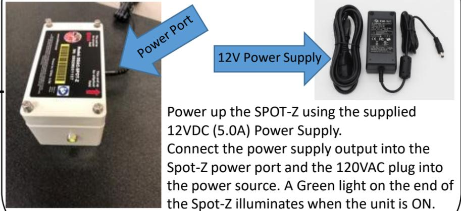
Power up the SPOT-Z using the supplied 12VDC (5.0A) Power Supply. Connect the power supply output into the Spot-Z power port and the 120VAC plug into the power source. A Green light on the end of the Spot-Z illuminates when the unit is ON.
