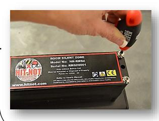
Remove the cover to the Room Silent Zone using an appropriate Phillips head screwdriver The unit will need to remain plugged in (Powered) while making the adjustments.
