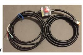
The cable exiting the warning module with the connector goes to the Generator
