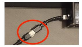
Connect Warning Module (Plug) to Generator (Receptacle).
