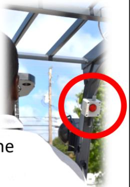
Place magnet side of the Warning Module to the frame of the forklift where it can be seen and heard by the operator. **Volume** can be reduced by turning the clear plastic cap.
