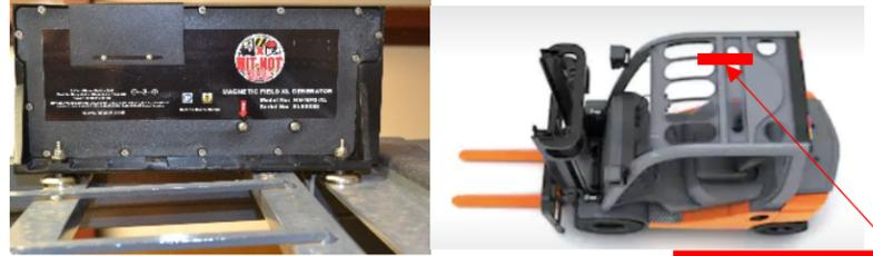
Install the Generator on top of the overhead guard or at least 4" from the frame if placed on the counterbalance. It should be as far from the strobe light as possible. Adjust magnets to fit as needed.
